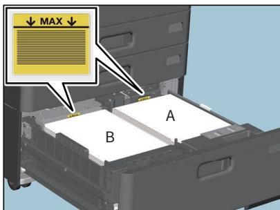
Fan and jog the paper well before placing it. Place it with its copy side up. Place one stack of paper in the right-hand tray (shown as “A” in the figure) with its side touching the right corner of the tray, and place the other stack of paper in the left-hand tray (shown as “B” in the figure) with its side touching the left corner of the tray. Paper can be placed neatly if you divide stacks into small bundles and pile them up on the two trays alternately.
