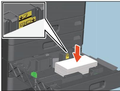
Load an envelope with its bottom side at the rear and its flap side at the front. If the flap of the envelope touches the side guide, fold the flap and load the envelope.
