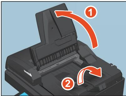
For using the DSDF, pull it out from the DSDF and raise the sub-stopper. If you do not raise the sub-stopper, paper misfeeding may occur depending on your paper or the exited originals may fall off the exit tray.
