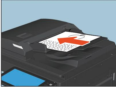
The original is automatically pulled in and then the menu of step 3 will be displayed on the touch panel.
