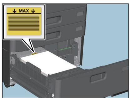
**3 Push the drawer of the Large Capacity Feeder straight into this equipment carefully.**
