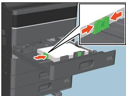
**6 Check that there is no gap between the paper and the side guides, as well as the paper and the end guide.**
